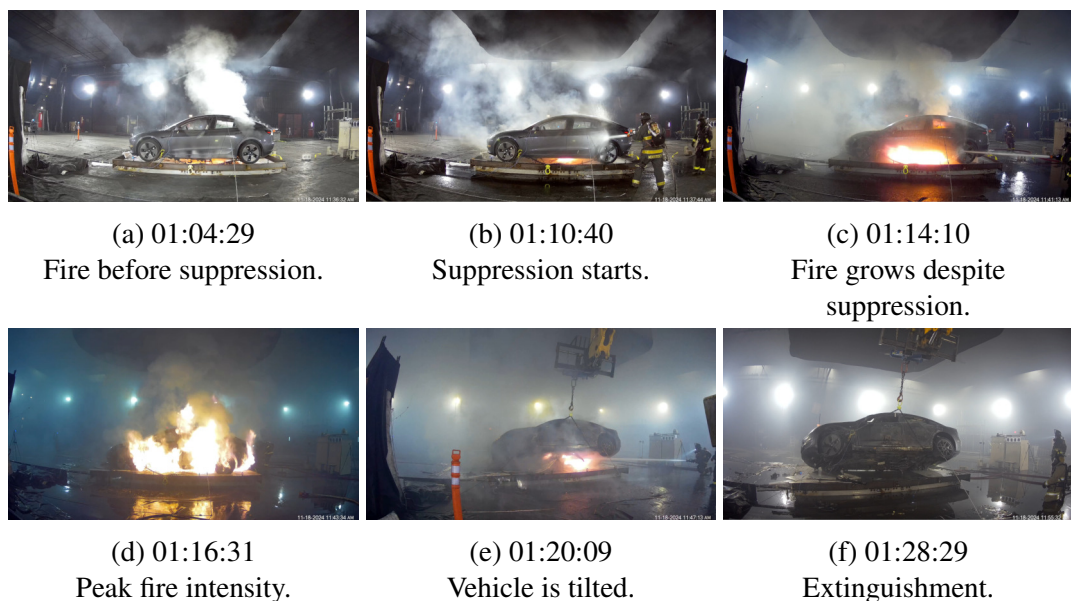
Figure 4.4: Timeline of experiment E-TM-S, time is in hours minutes and seconds since ignition.
