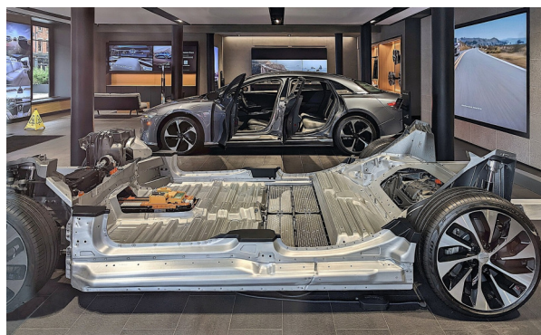
(b) Structural integration of battery pack [95].
