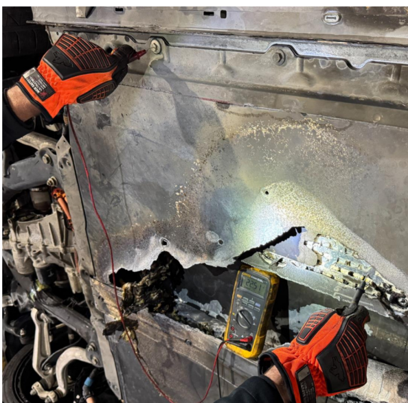
(b) The current collector in E-TM-S was readily exposed posing a potential electrical hazard.
