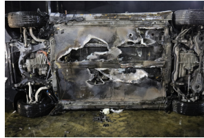
(h) Battery Damage for E-TM-S.
