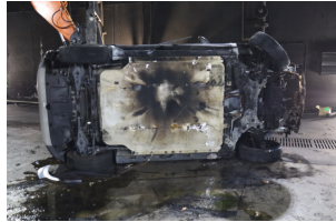
(f) Battery Damage for E-HK-S.
