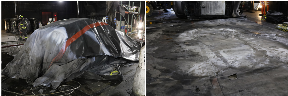
(a) Discoloration visible on the applied blanket, E-TM-BS.
