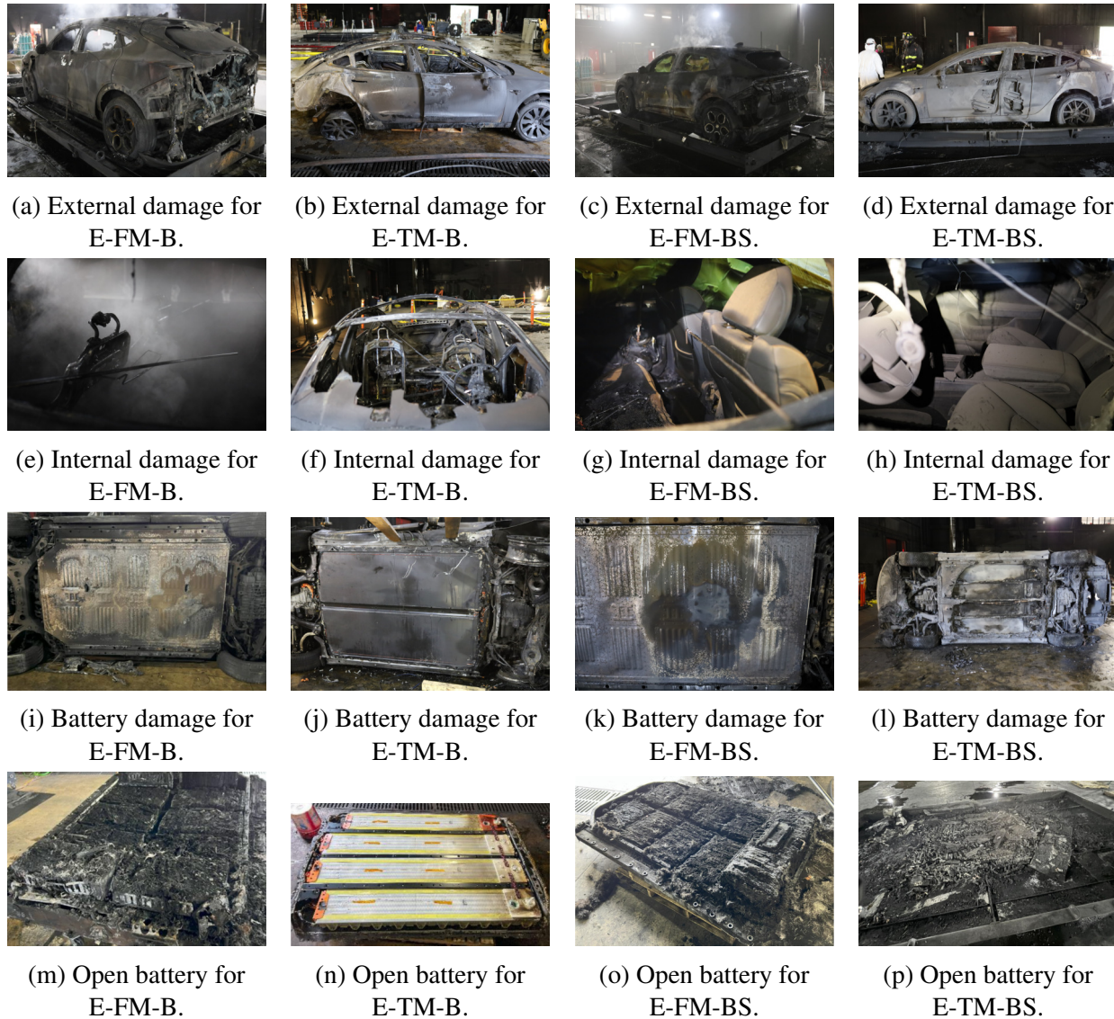
Figure 4.19: Damage patterns for the EV fire blanket experiments.
