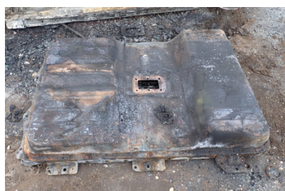
(a) Steel case battery pack after fire test.
