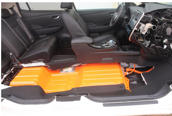
(a) Non-structural integration of battery pack [94].
