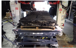
(g) Battery Damage for E-CB-S.
