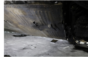
(j) Battery Damage for E-FM-SA.
